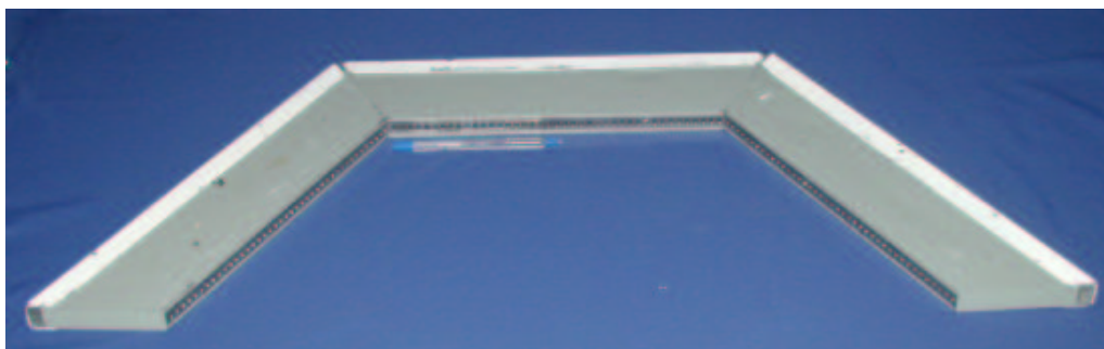
Figure 1.3: Three 6P-SPECT collimators. If TLDs would be used as radiation detectors, all projections could be measured simultaneously.
